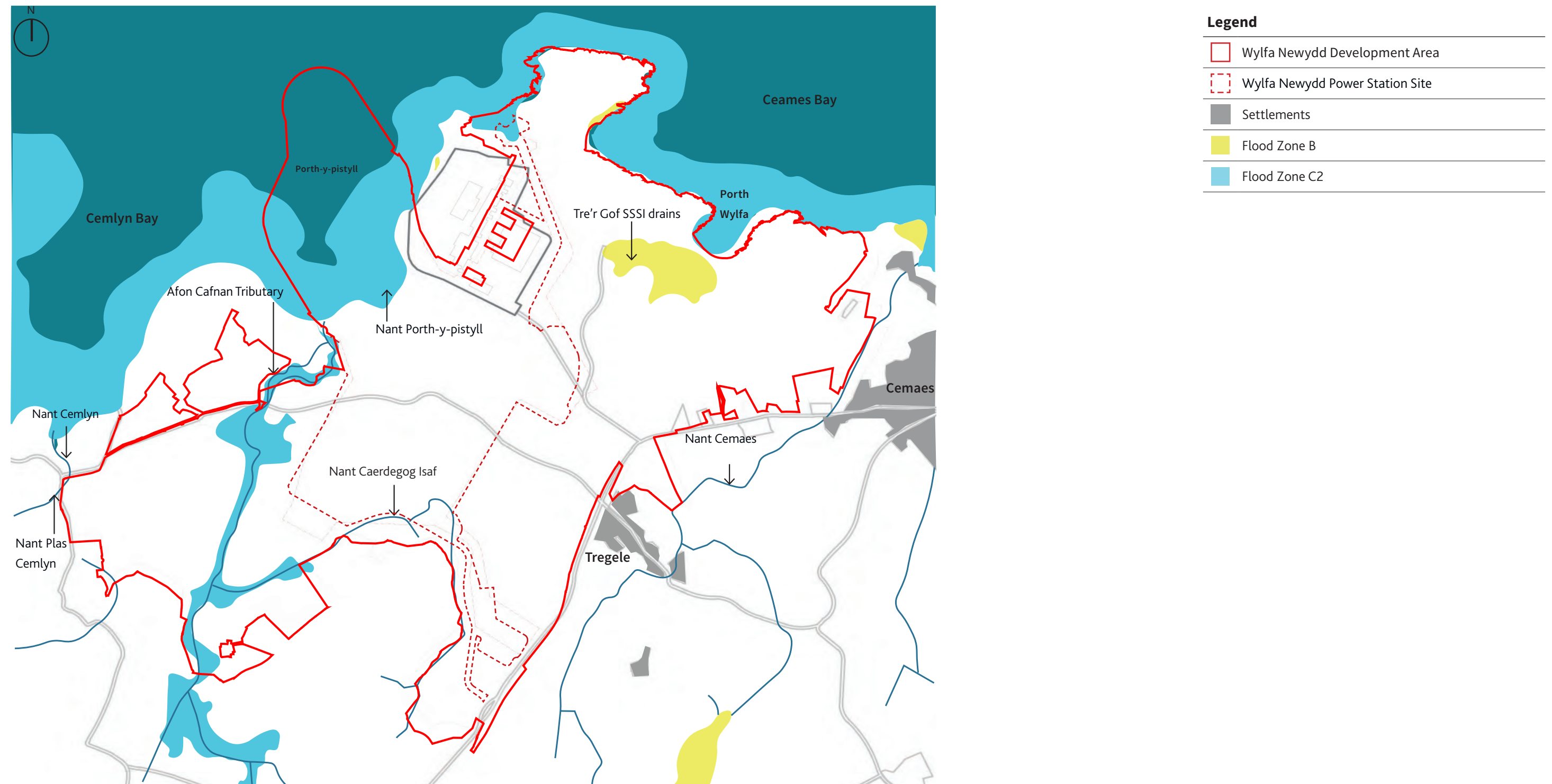
Figure 2-17 Risk of flooding from rivers and sea
