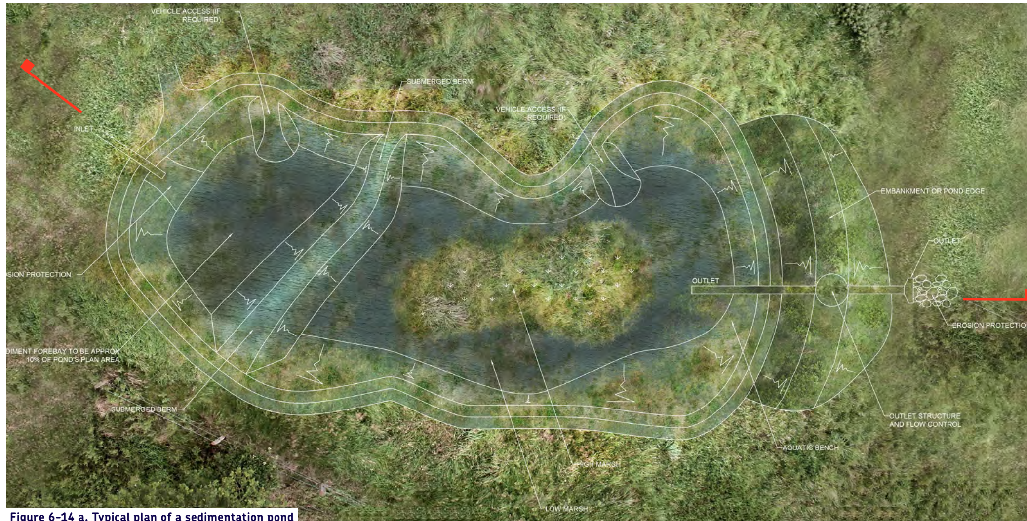
Figure 6-14 a. Typical plan of a sedimentation pond
